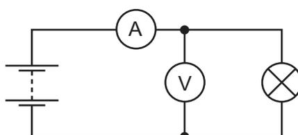
The lamp is a 12W lamp and is working at normal brightness.
